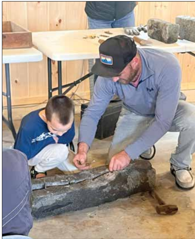
Joe (right) and his son Leo (left) demonstrating how to split a rock with shims and wedges.
