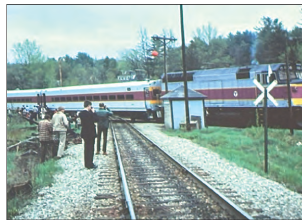
The lowering of the ball signal at Whitefield.
